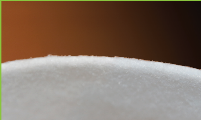
Synthetic felts provide depth filtration and higher solid loading capacity than comparable mesh fabric bags.
