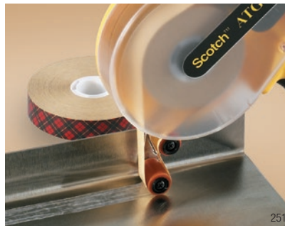
Save time and effort with Scotch® ATG Transfer Tapes and Applicators. You apply a precise strip of adhesive at the same time as the liner rewinds into the applicator.
